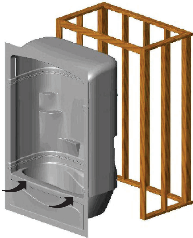
FIGURE 3 - POSITION TUB SHOWER UNIT IN FRONT OF FRAMING
